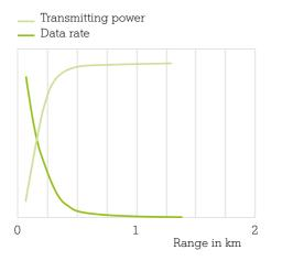
Transmitting power, data transfer rate and range of an LTE-2,600 MHz base station
