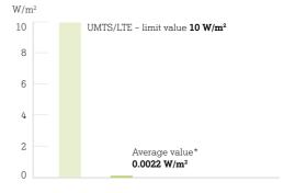
Result of the test series for UMTS frequency ranges by the Austrian Ministry for Transport, Innovation and Technology
