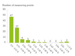
A nationwide LTE measurement by IZMF in Germany shows: The measured values at all measuring locations are far below the WHO limit value of 10  $W/m^2$
