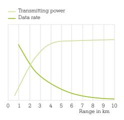
Transmitting power, data transfer rate and range of an LTE-800-MHz base station
